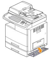
**3** Pull the jammed paper out in the direction shown. To avoid tearing the paper, pull it out gently and slowly.
